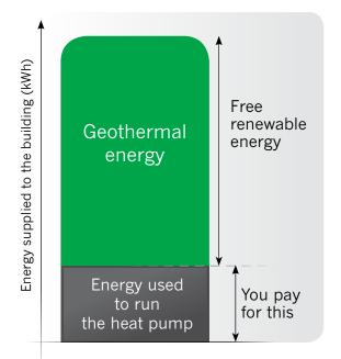
This graphic shows the building's total energy consumption for heating and hot water. The grey area shows the energy used to run the heat pump. The calculation was made for a building of 1 000 m<sup>2</sup> in an average weather year.
